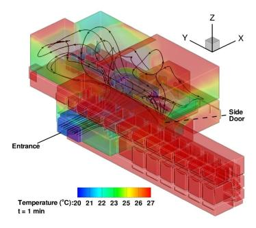
Figure 5: Internal air flow pattern at Viipuri library
