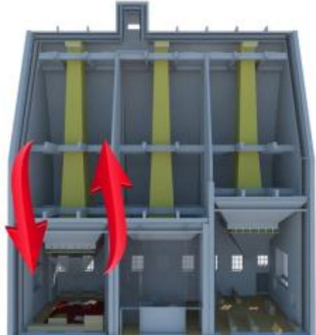
9.-10. Design proposal for the ex-chip container: a Multi-faith space – images: Francesca Paola Piccolo The modules are divided by flexible glazed surfaces. Each module can works independently or together, creating different functional combinations. The hoppers are connected to cones and hide the controlled mechanical ventilation. The cones are “stretch ceilings” with lighting diffusers .
