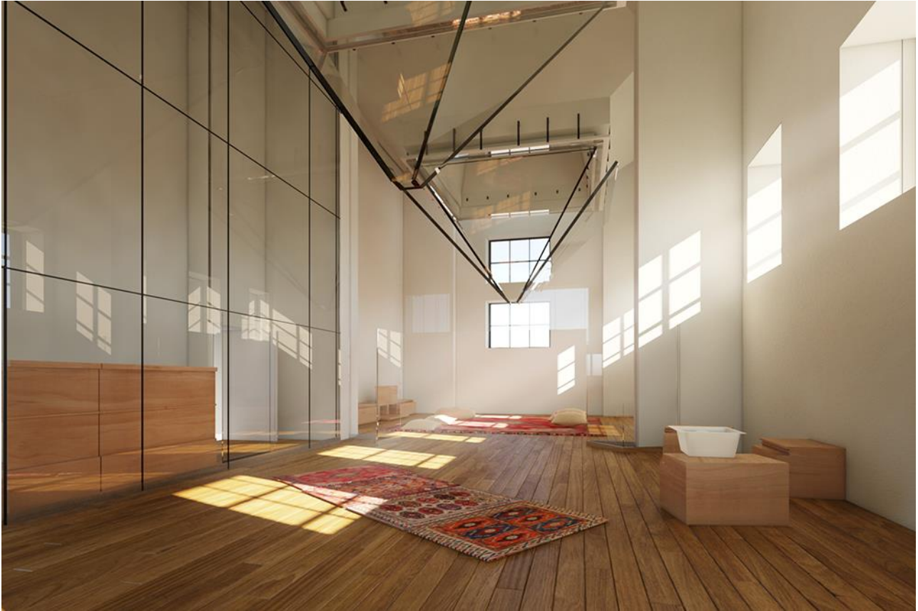
8. Design proposal for the ex-chip container: a Multi-faith space – image: Francesca Paola Piccolo The original hoppers has been removed to ease the ventilation and to unload the structure. The new ones are light, transparent, openable and removable: they aim at keeping the same spatial quality. Dry assembly solutions for the internal insulation finishing system and radiant floor panels.
