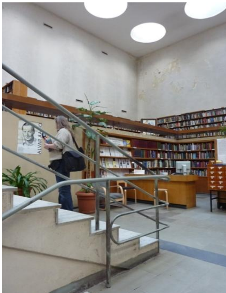
Vyborg Library interior. Grills for supply and exhaust ventilation dissipate into the smooth walls. Photo Seija Linnanmäki 2010.
