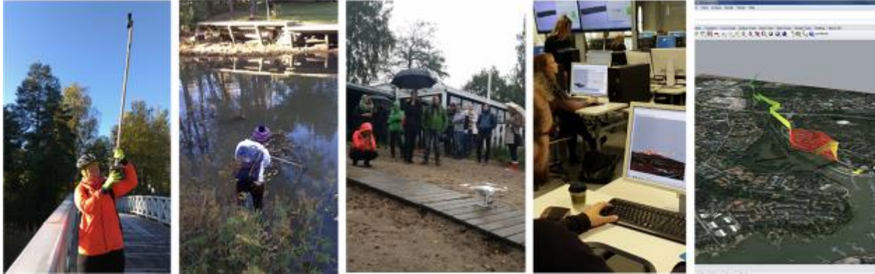
Fig. 3 Field work of students of the Department of Architecture: Integration of sensor data (wind, noise and water quality). This data was integrated through a grasshopper script into the design process and overlayed with high-resolution data from the site, generated from a point cloud.
